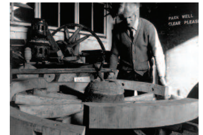
Cyril Sissons wheelwright from Beswick demonstrates making a wheel.
